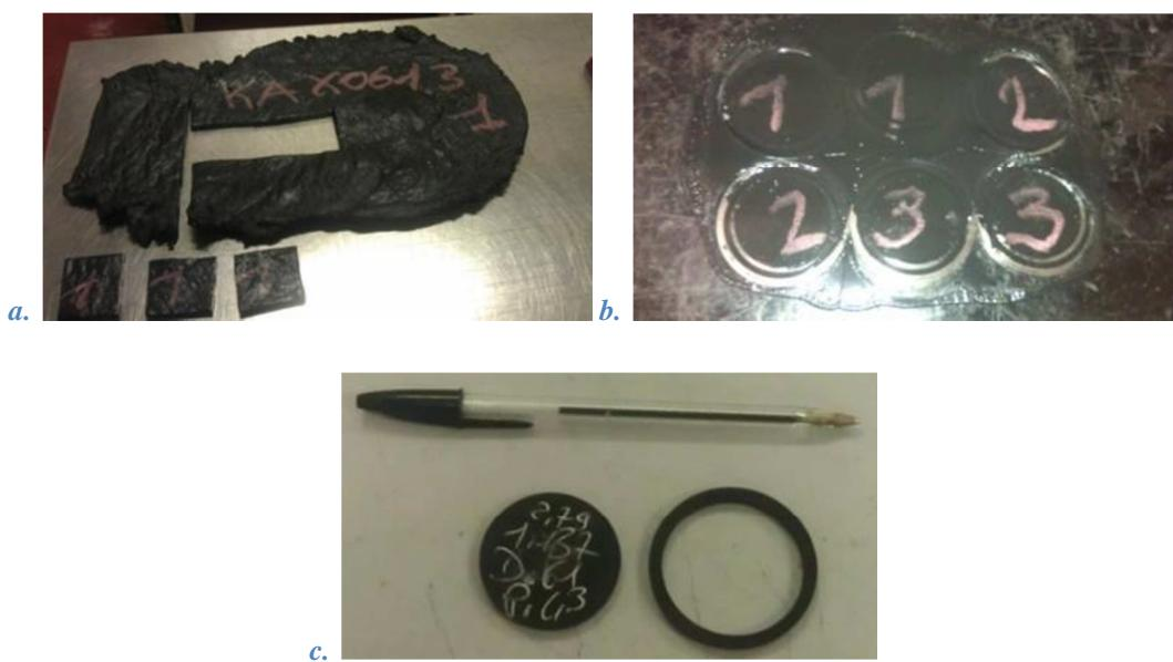
**Fig. 2.** Final batch; b. Stamp-vulcanized samples; c. Disk-shape compound and O – Ring specimen.
