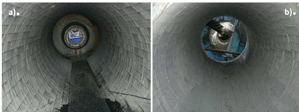
**Figure 6 Wear conditions after 1,25Mt discards washing: a) I stage; b) II stage**
