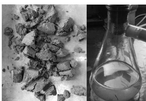
**Fig. 8: Tailings filter cake and filtrate produced using Invoque®**
