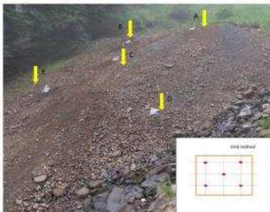
Figure 2 : Typical rock waste dump. The adopted sampling grid is also shown.
