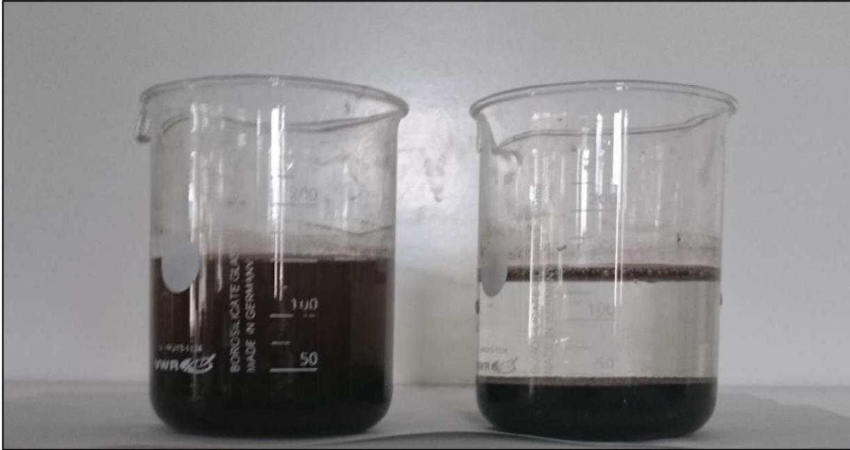
Fig. 3 Visual assessment of control versus conditioned sample after 5 minutes
