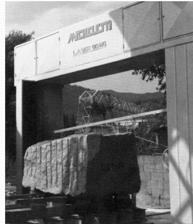
Micheletti Laser 90 MG sawing a red granite block (fonte: Daniel, 1986).
